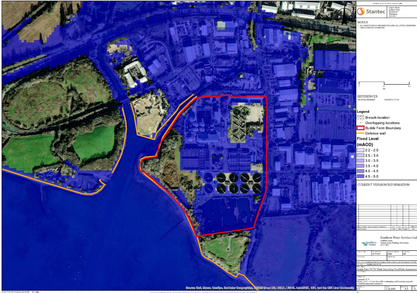
Figure B.2: Projected flood level for the credible maximum climate change scenario in proximity of Budds Farm WTW
