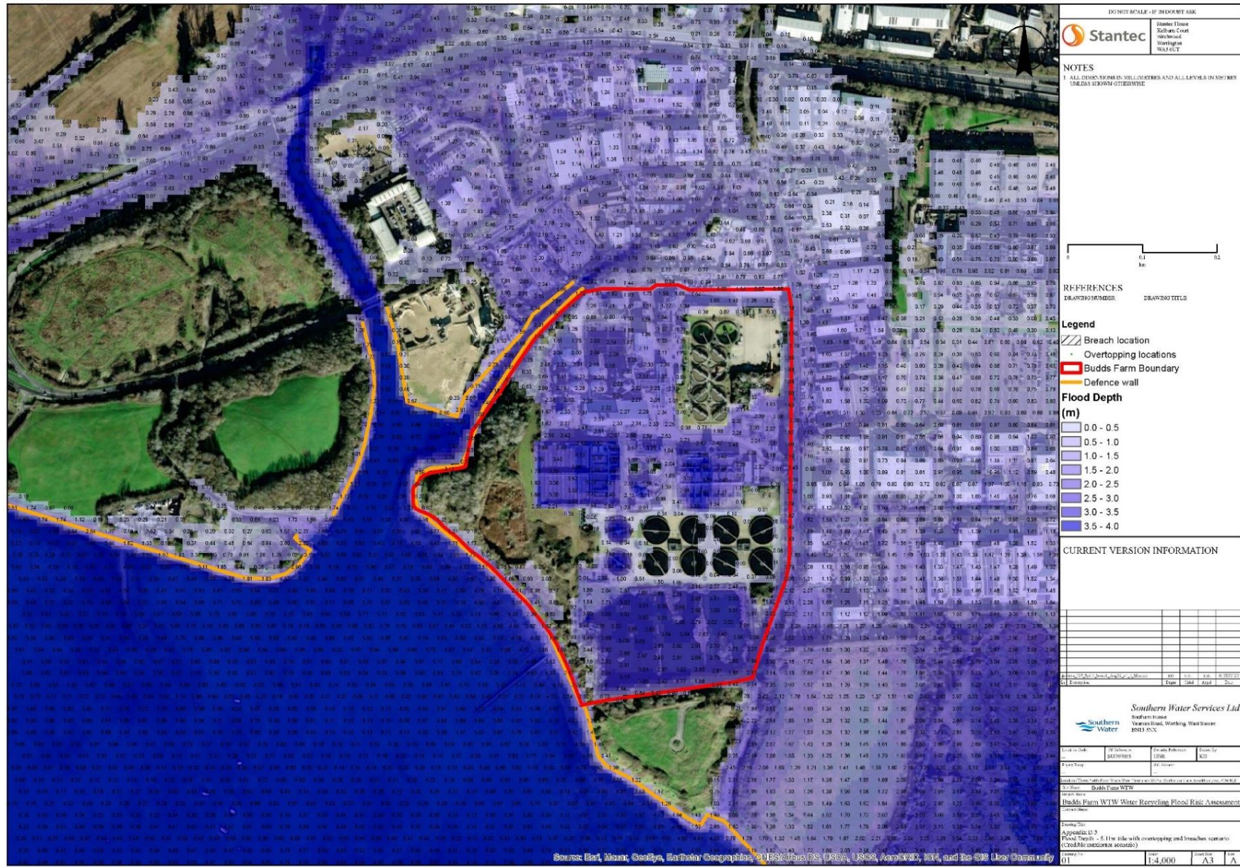
Figure B.1: Projected flood depth for the credible maximum climate change scenario in the proximity of Budds Farm WTW
